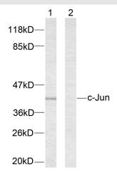
Western blot analysis of extracts from NIH/3T3 cells treated with UV. Line1: Using c-Jun(Ab-63) Antibody; Line2:The same antibody preincubated with synthesized peptide.
